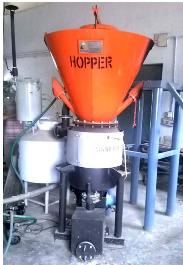
Fig. 1: Downdraft gasifier system coupled to the gas cleaning system
